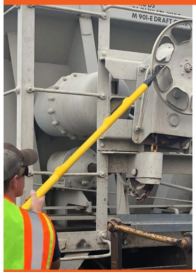
**NEW, LIGHT-WEIGHT TECHNOLOGY** creates a single handle tool used to push or pull brake wheels, push brake release levers, turn angle cocks, adjust draw bars, and arm EOTS.
